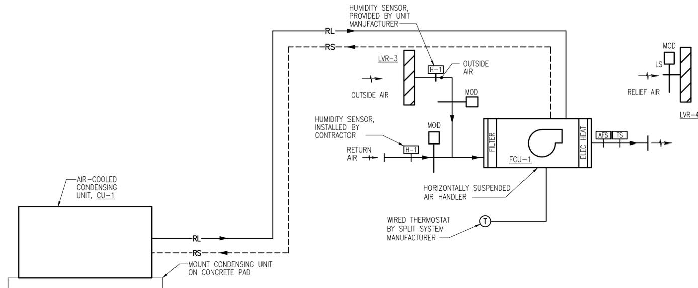
1 EQUIPMENT ROOM SPLIT SYSTEM CONTROLS SCHEMATIC
