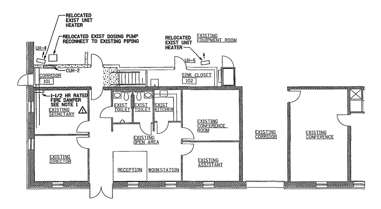
NOTES: 1. FIRE DAMPERS SHALL BE TYPE B AND HAVE A MAXIMUM AIR VELOCITY AND STATIC PRESSURE RATING SUITABLE FOR USE IN THE INSTALLED AIR SYSTEM. FIRE DAMPERS SHALL UL-555 LISTED. PROVIDE ACCESS DOOR FOR INSPECTION OF FIRE DAMPER.
