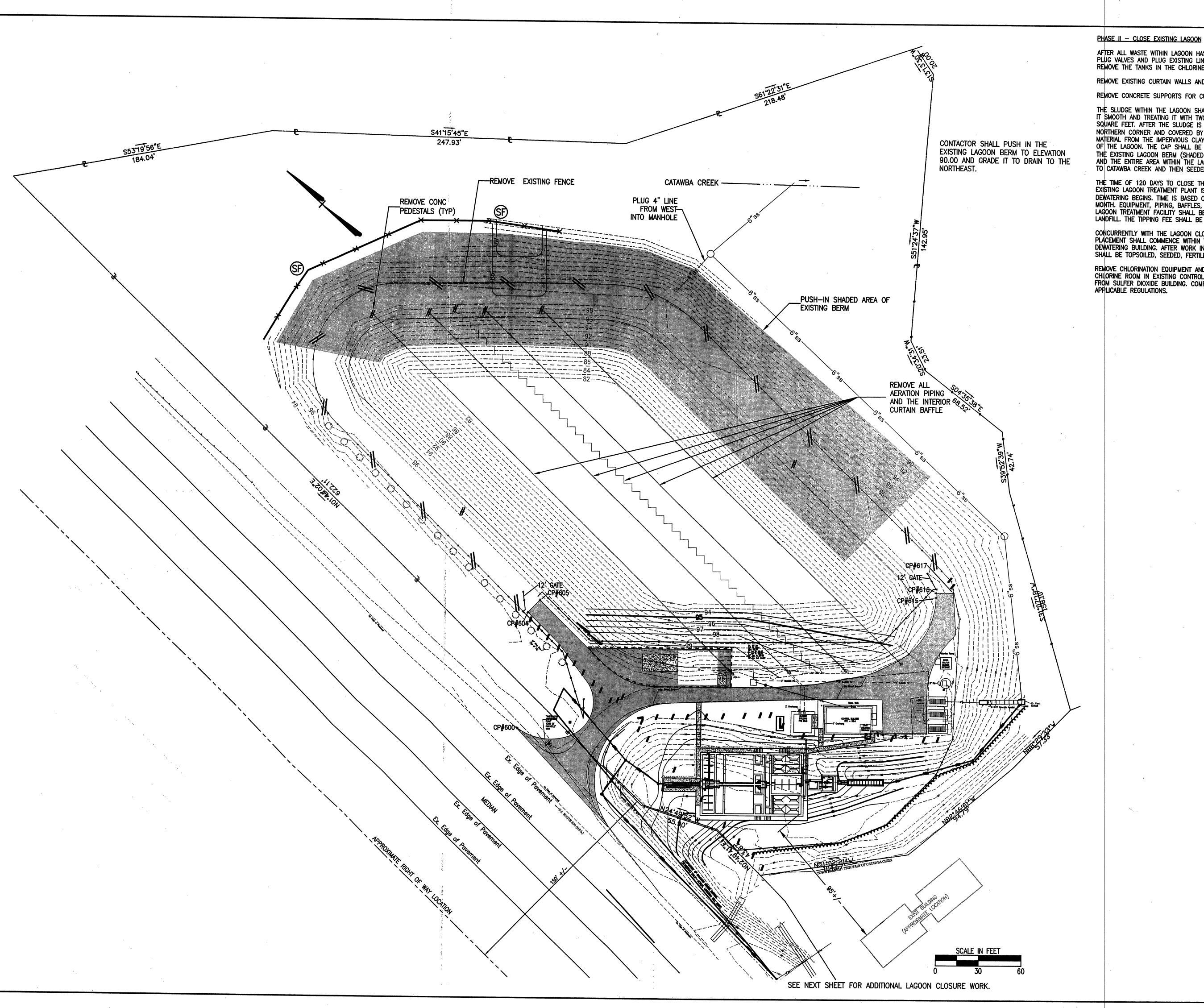
AFTER ALL WASTE WITHIN LAGOON HAS BEEN PROCESSED, CLOSE ALL PLUG VALVES AND PLUG EXISTING LINES WHICH ARE TO BE ABANDONED. REMOVE THE TANKS IN THE CHLORINE ROOM.
