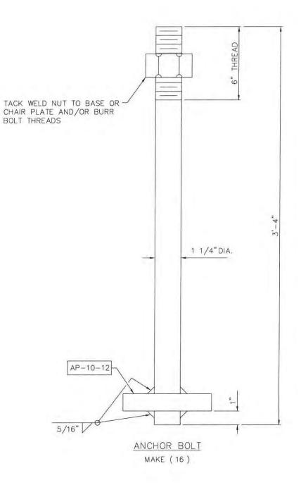
STEEL: ASTM A36 FINISH: NONE
